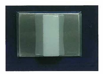
The corridor light is available with 1, 2, or 3 lamps furnished with steel segment dividers for individual light separation. The shatter proof, wedge-shaped translucent dome snaps into a stainless steel face plate for ease of lamp replacement and concealment of mounting screws.
