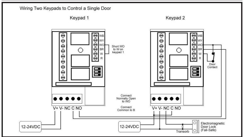
The diagram above shows how to connect two keypads to control a single door. Entering your code on keypad 2 unlocks the maglock directly. When you enter your code on keypad 1, it triggers the REX input of keypad 2, which unlocks the door.
