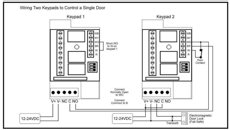
The diagram above shows how to connect two keypads to control a single door. Entering your code on keypad 2 unlocks the maglock directly. When you enter your code on keypad 1, it triggers the REX input of keypad 2, which unlocks the door.
