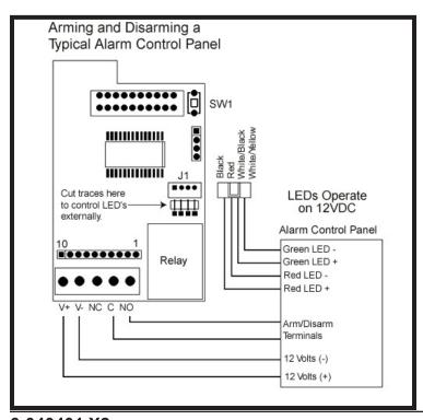
The diagram to the left shows how to control the keypad LED's using an external alarm panel. To access the keypad's main circuit board, remove the relay board.
